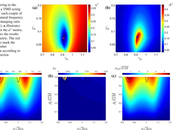
Fig. 6 System response for a TMD acting in heave, tuned according to the optima in Fig. 5a ( $\varepsilon = 0.05$ ,  $\gamma_a = 0.9125$  and  $\zeta_a = 0.074$ ). Colours indicate: **a** normalized heave  $(x_3/\overline{GM})$ ,
