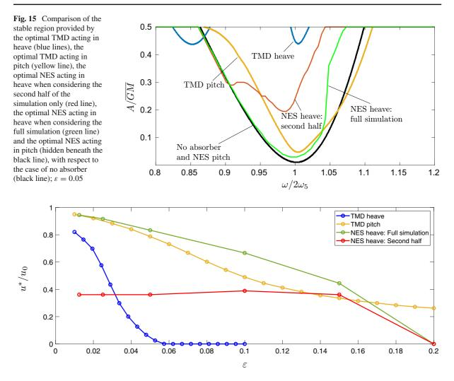
Fig. 16 Minimum parametric resonance region ratio,  $u^*$ , achievable for the different DVA configurations for varying mass ratio values,  $\varepsilon$ , normalized against the parametric resonance region ratio for the baseline case with no absorber ( $u_0^* = 0.36$ )
