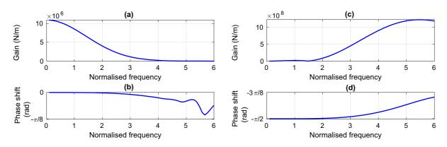
**Fig. 2** Excitation force coefficients **a**  $H_{E,3}(\omega)$ , **b**  $\phi_{E,3}(\omega)$ , **c**  $H_{E,5}(\omega)$  and **d**  $\phi_{E,5}(\omega)$
