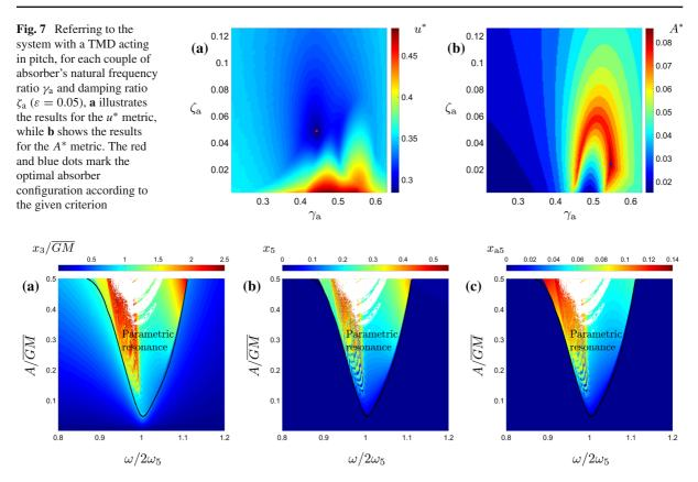
**Fig. 8** System response with a TMD in pitch, tuned according to the optimization in Fig. 5a ( $\varepsilon = 0.05$ ,  $\gamma_a = 0.4427$  and  $\zeta_a = 0.0487$ ). Colours indicate: **a** normalized heave  $(x_3/\overline{GM})$ , **b** pitch ( $x_5$ ) and **c** absorber displacement ( $x_{a5}$ ). The thick black
