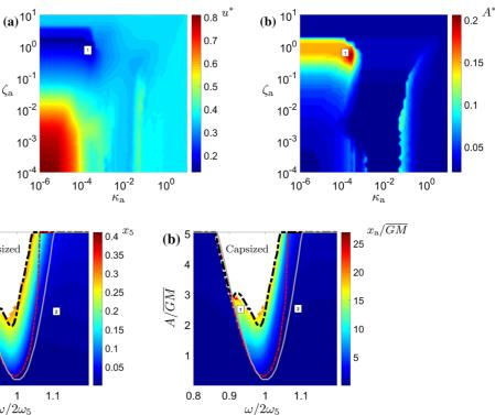
ering the second half of the time series by the black dashed line. For reference, the baseline region of parametric resonance, for the case with no DVA, is denoted by the solid grey line. The white area indicates where the pitch angle exceeded 90 degrees and the simulation was aborted
