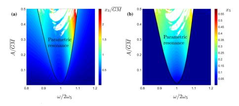
Fig. 4 Frequency/amplitude range of input waves considered for the analysis of the generation of parametric resonances. Regular resonance solutions are generated through the HBM, while parametric resonances through direct numerical simulations. Colours
