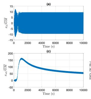
**Fig. 13** Simulation results from Point 1 in Figure 12 ( $A/\overline{GM} = 0.26$ ,  $\omega/2\omega_5 = 0.93$ ) **a** The normalized heave motion **b** The pitch motion **c** the normalized DVA motion **d** The pitch motion
