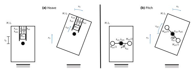
Fig. 3 Schematic of the DVA attachment to the cylinder for a the heave DoF and b the pitch DoF
