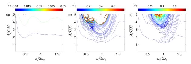
Fig. 20 Comparison of the maximum pitch displacement over the **a** TMD acting in heave using the parameters from point 1 in Fig. 18, **b** NES acting in heave using the parameters from point 1
