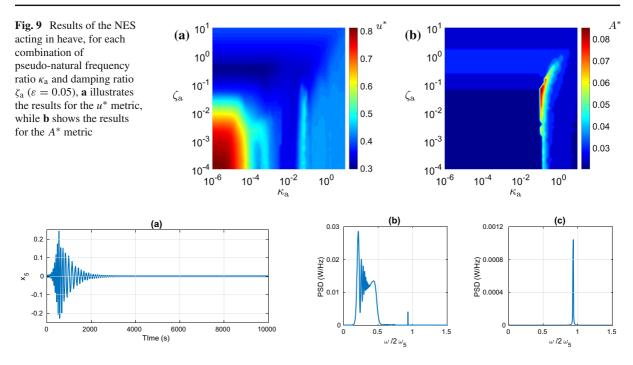
Fig. 10 Example of post process identification of PR: **a** The pitch displacement time series, **b** The PSD for the entire time series **c** The PSD for only the second half of the time series
