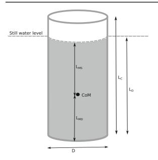
Fig. 1 Cylinder schematic with geometrical parameters utilized in the numerical model
